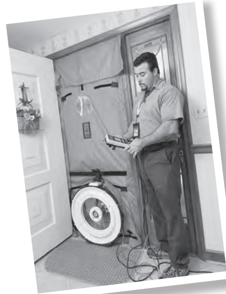
Blower door technology measures home air leakage.
